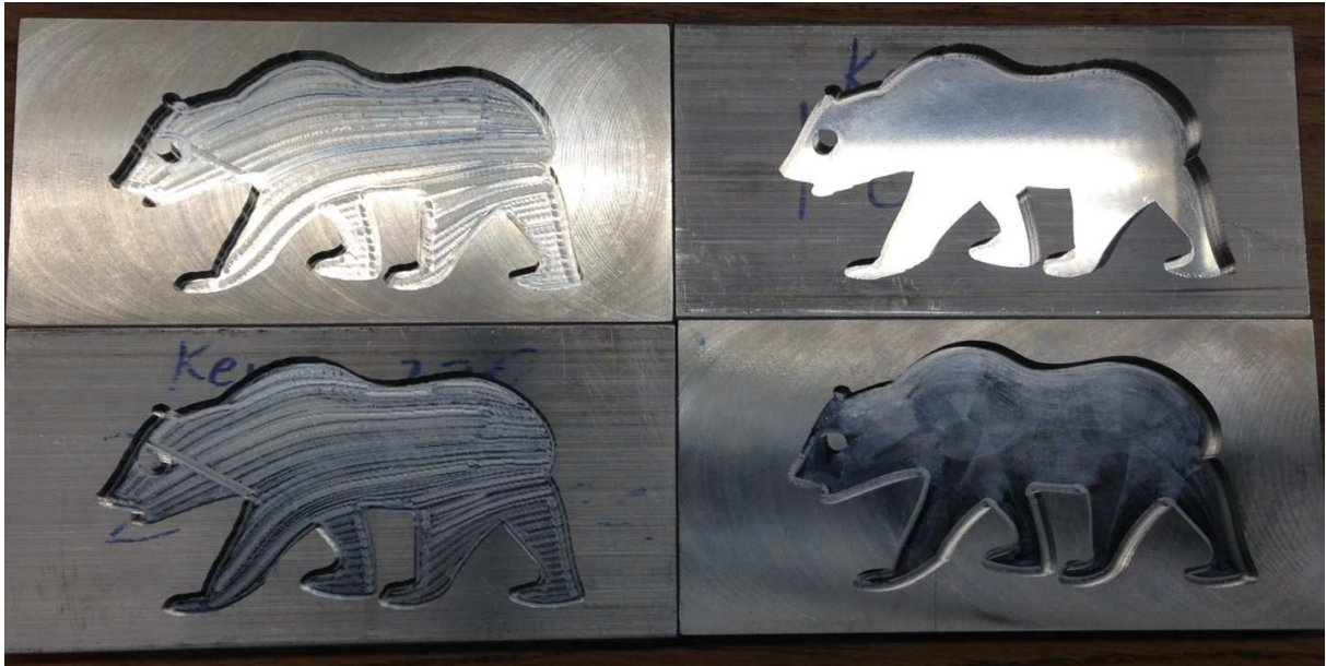
Figure 21: Raw surface finish for all four tool paths
