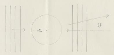
The wave scattered into the angle  $\theta$  (see Figure) will, therefore, result partly from a "forward" scattering of the waves coming from the left and a "backward" scattering of the opposite wave train, and the anomaly in the scattering law arising from the identity of the particles is simply that due to the interference of these two scattered waves.
