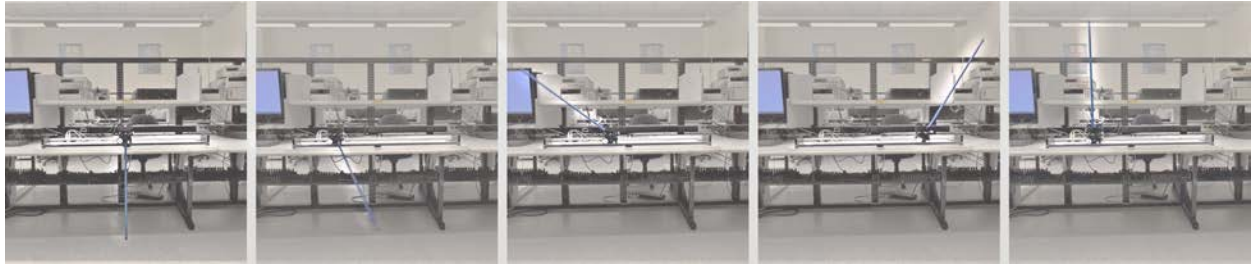
Figure 2.5: We learn precise stabilizing policies on hardware for the Quanser cartpole [84] using less than 20 seconds of data. A video of our experiments can be found here https://youtu.be/l7kBfitE5n8
