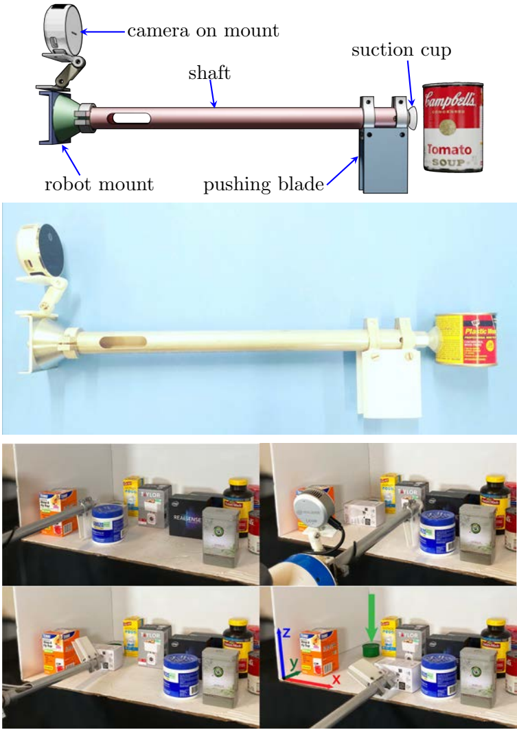
Figure 9.1: Bluction Tool : CAD (top) and physical implementation (middle). Using the bluction tool, the SLAX-RAY policy performs pushing and suction actions (bottom) to reveal the green cylinder target object among occluding objects within the shelf. Suction actions increase the robot search efficiency and can reveal the target object in scenes where no pushing actions are available. The shelf coordinate system is shown in the bottom right.
