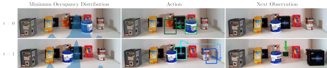
Figure 9.3: Bluction tool camera view with overlaid occupancy distribution and actions. At each timestep, Bluction-DAR computes the minimum of the predicted target occupancy distribution at the current timestep and that from the previous timestep (left, light blue overlay). It executes the pushing action (top, green) or suction action (bottom, blue) that maximally reduces the support area of the distribution. The dotted arrows represent the motion of the end-effector from the lighter colored box to the darker color. Suction actions are advantageous when moving objects that are very close. They follow the piecewise linear trajectory described in Sec. 9.2, as in the bottom row.
