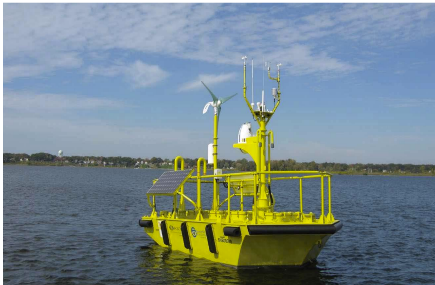
Figure 3.1: One of the two AXYS WindSentinel LiDAR buoys operated by the Pacific Northwest National Laboratory (PNNL) for DOE. The LiDAR instrument is the small white cube atop the platform on the large mast. (Image from BOEM.gov)
