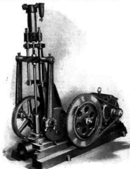
"Reeco" Deep Well Head. Capable of pumping from wells 50 to 500 feet deep.
