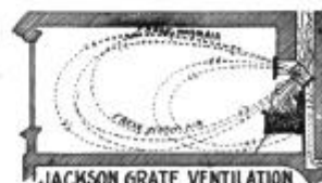
JACKSON GRATE VENTILATION SHUTS OUT COLD AIR CURRENTS
