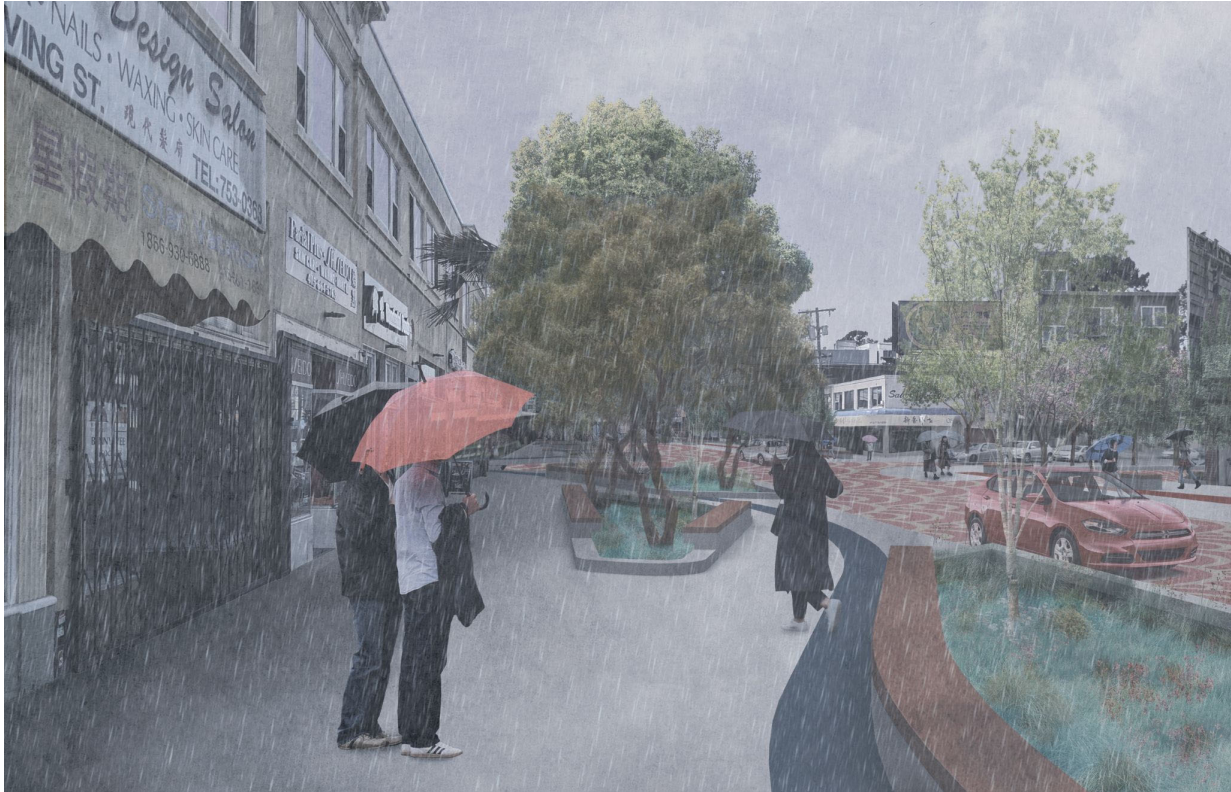
Figure 5.22 Water element as the park-like streetspace, with planters at capacity during an intense storm.
