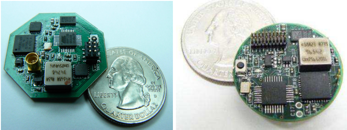
Figure 2.2: GINA 0 on the left and GINA 1 on the right were created to guide small scale rockets and designed to be the smallest and lightest inertial flight controllers.
