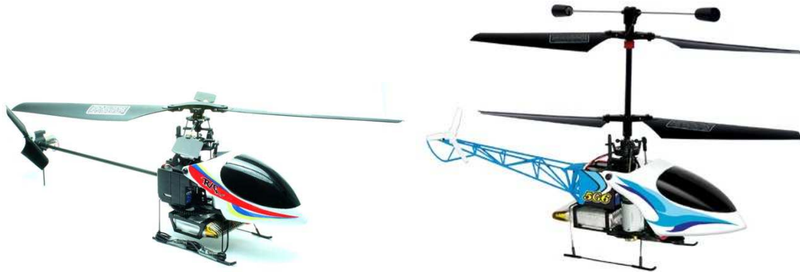
Figure 3.8: The Walkera helicopters selected as the platforms for this project are small, cheap, and commercially available 4 channel electric helicopters.
