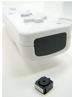
Figure 3.16: The commercially available WiiMote contains a 300 mg “smart camera,” which contains image processing hardware to return the coordinates of IR blobs in its field of view.
