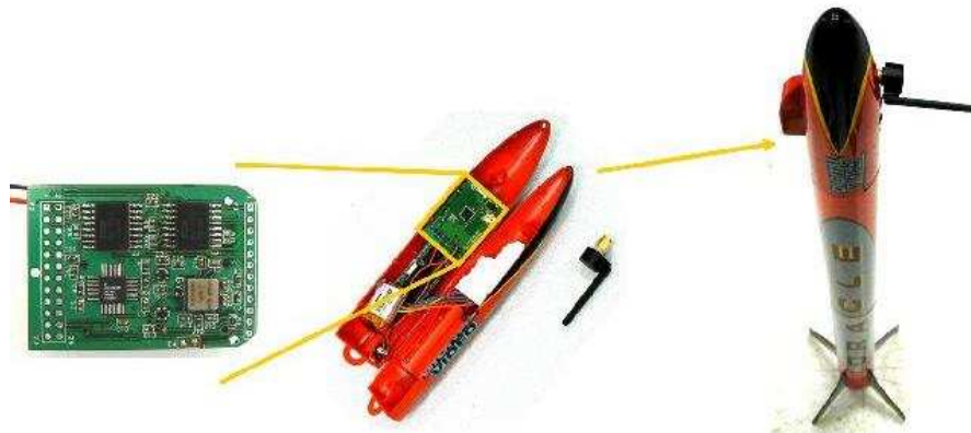
Figure 3.3: The original rocket containing GINA sensors and a video camera
