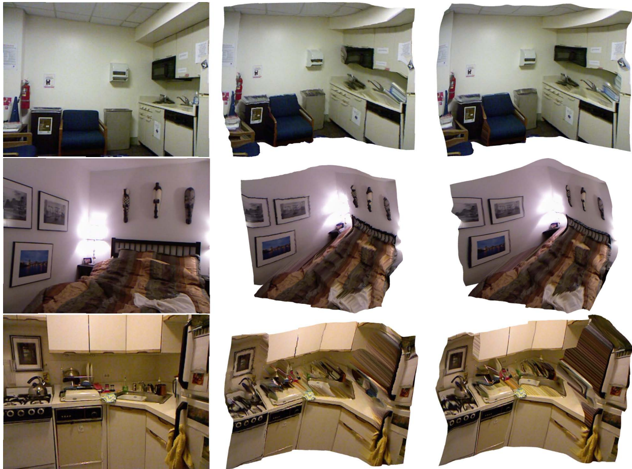
Figure 3.8: After a model is recovered, the camera can be moved and the input image (left) can be shown from a different viewpoint (right). Such a warping could be produced using just the smoothed Kinect depth maps provided in the NYU dataset (middle), but these images have jagged artifacts at surface and normal discontinuities. Both renderings, of course, contain artifacts in occluded regions.
