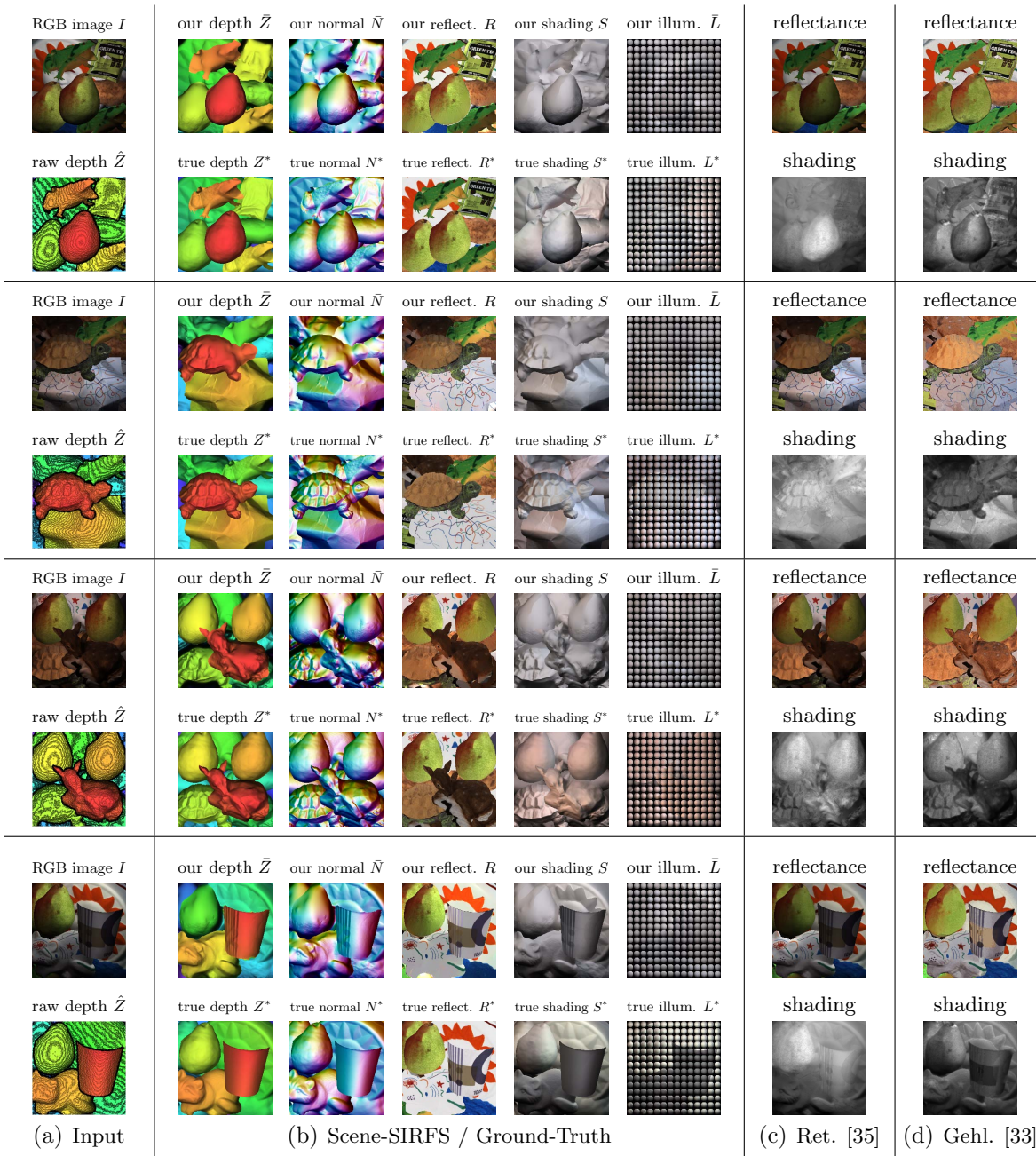
Figure 3.4: A test-set scene from our pseudo-synthetic scene dataset. In 3.4(a) we have the input to our model: an RGB image and a noisy Kinect-like depth map. In 3.4(b) we have the depth map, surface normals, reflectance, shading, and spatially-varying illumination that our model produces, and the corresponding ground-truth scene properties on the bottom. In 3.4(c) and 3.4(d) we show the shading and reflectance images produced by the best-performing intrinsic image algorithms. See the supplementary material for additional similar figures.
