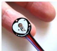
Figure 9. Open source optical sensor sold by Joel Murphy and Yury Giyman
