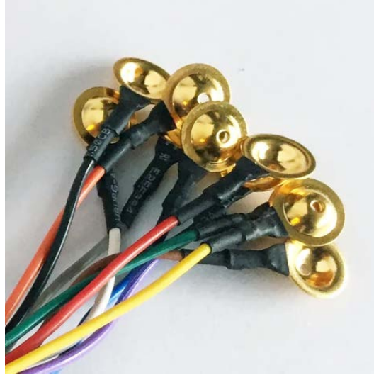
Figure 2.1: Gold-plated cup electrodes used for capturing EMG.
