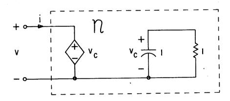
Figure. An example of a one-port electrical network  ${\cal N}$  which is active and uncontrollable.
