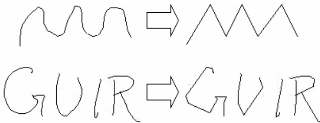
Figure 7 – Two examples of stroke simplification. The algorithm generates a stroke similar to the original stroke, but has fewer points and can thus be rendered faster.
