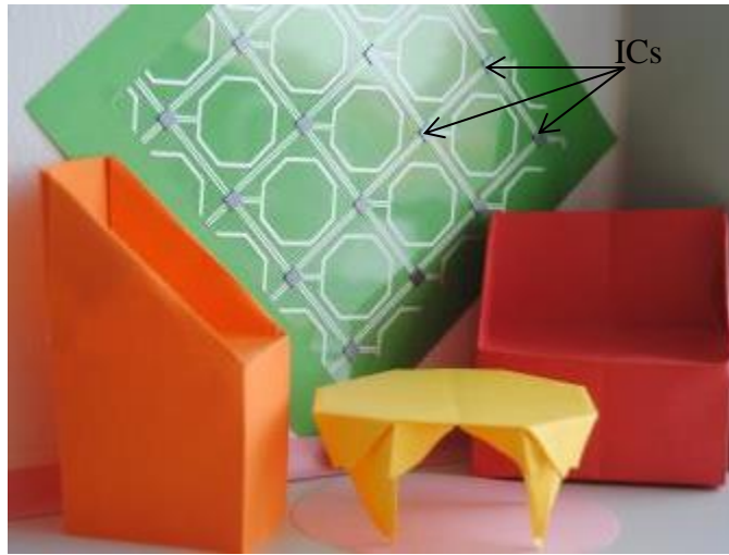
Fig. 1. Electronic wallpaper (a two-dimensional distributed network of silicon ICs, spaced 25 mm apart, and screen-printed antennas) in a living room setting
