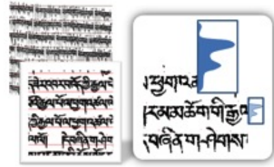
Fig. 9. Baseline detection using horizontal histograms
